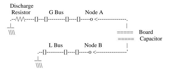
If the board capacitor is connected to a fixed node on either end, the L Bus will be automatically be connected to the capacitor node closest to ground (from software revision B2.50 on, see Appendix A).
